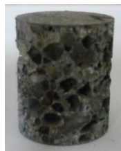
Figure 4.9. Al foam test sample with SiC particles.
