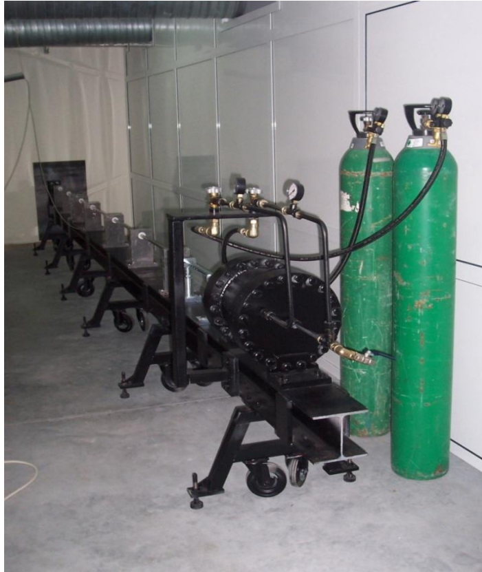
Figure 4.2. SHPB apparatus in DTM Lab at IZTECH.
