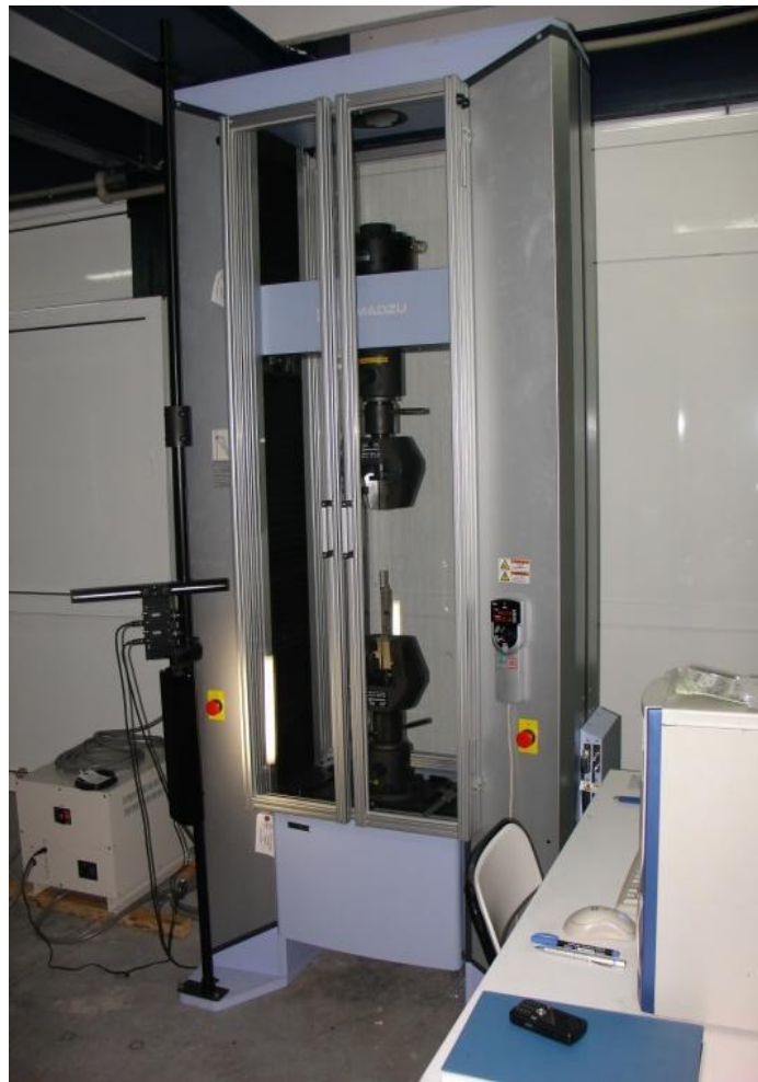
Figure 4.1. Static test machine (SHIMADZU AG-300kNX).
