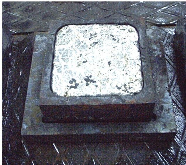
Figure 4.8. Foamed precursor that completely filled foaming the mold.
