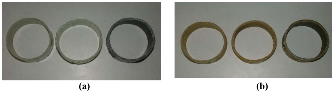
Figure 6.48 Photos of the mechanical testing specimens of tube rolled composite tubes loaded along radial direction and exposed to (a) dry environment (b) geothermal fluid.
