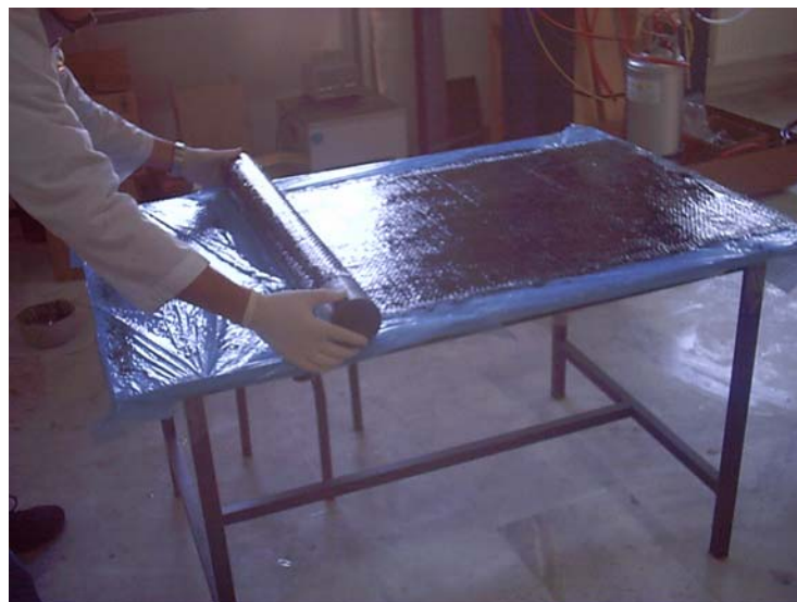
Figure 5.5 Rolling of pre-impregnated fiber on the mandrel.
