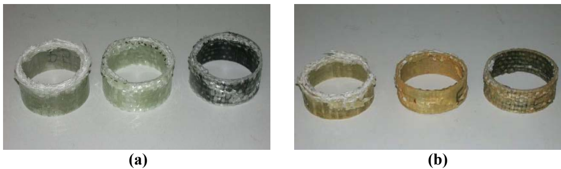
Figure 6.47 Photos of the mechanical testing specimens of tube rolled composite tubes loaded along axial direction and exposed to (a) dry environment (b) geothermal fluid.
