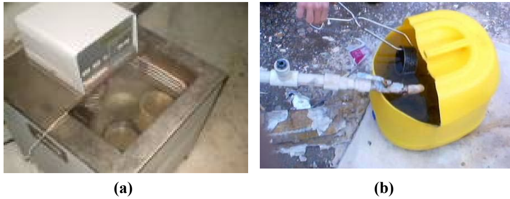
Figure 5.6 (a) Distilled water tank and (b) geothermal fluid bath with continuous flow.
