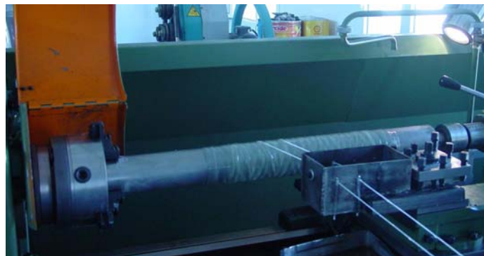
Figure 5.2 The experimental setup (filament winding machine).
