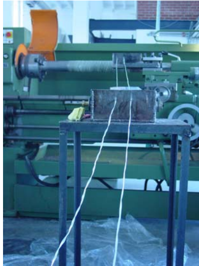
Figure 5.3 The experimental setup (resin bath).
