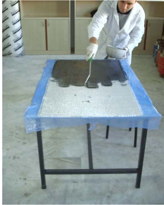
Figure 5.4 Pre-impregnation of the fiber.
