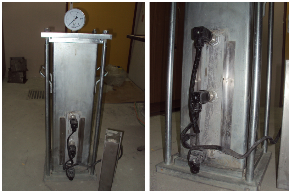
Fig. 4. Steel pressure formwork.
