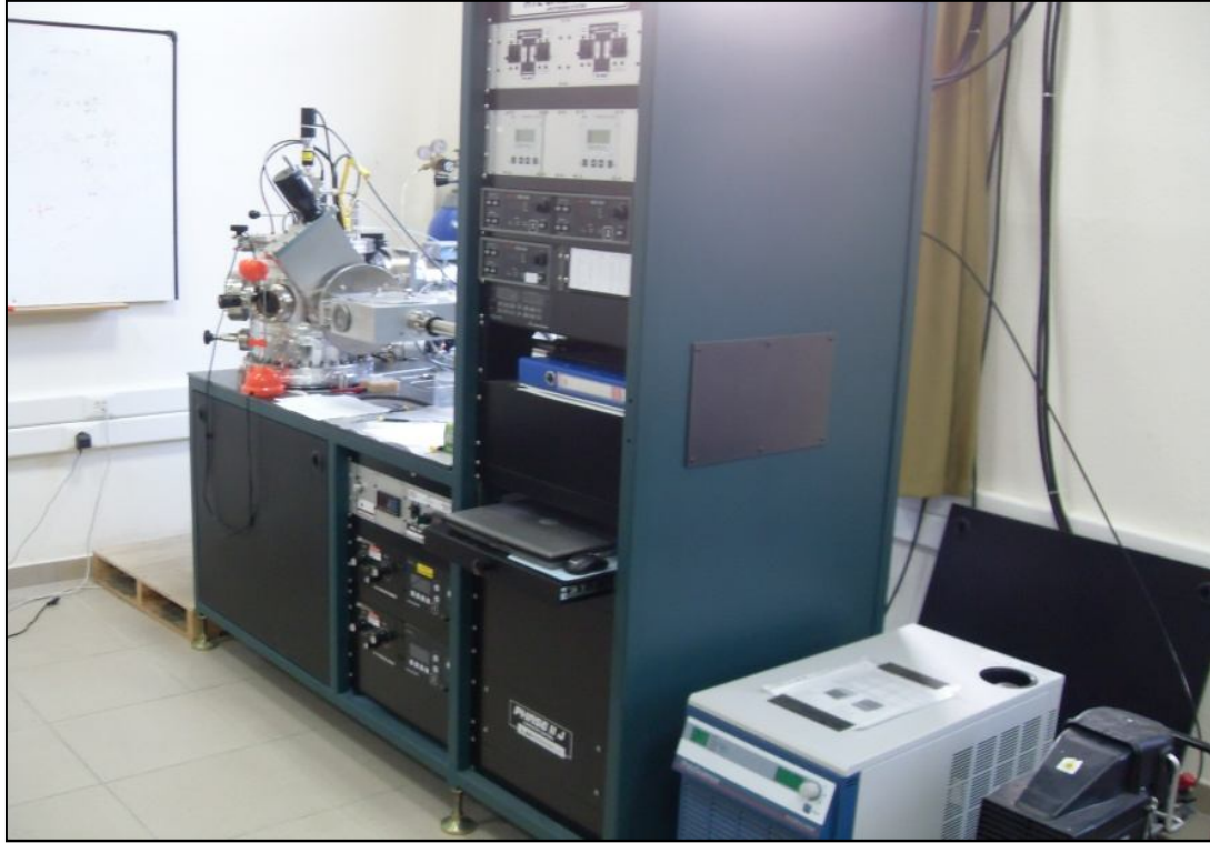
Figure 3.2. ATC ORION 5 UHV Magnetron Sputtering System.
