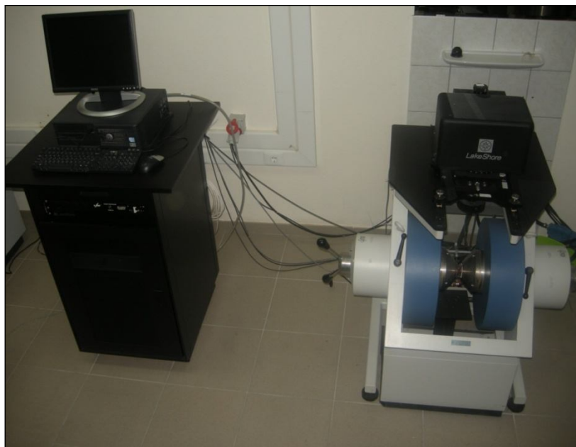
Figure 3.11. Lakeshore 7400 Vibrating Sample Magnetometer (VSM).
