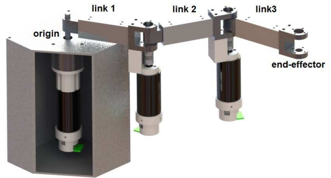
Fig. 5. The 3 degree of freedom robot manipulator
