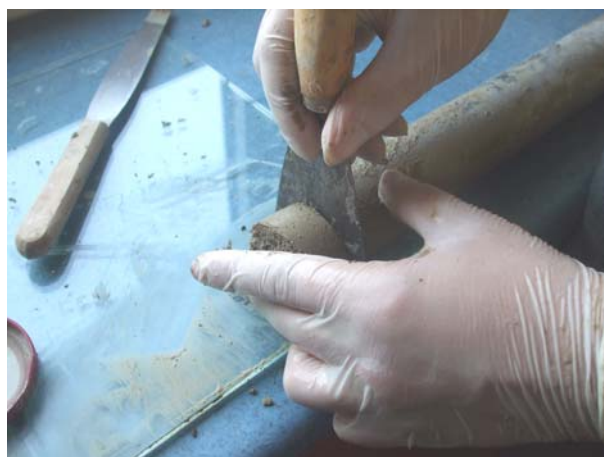
Figure 4.31. A View from how 3cm High Soil Subsample is Obtained
