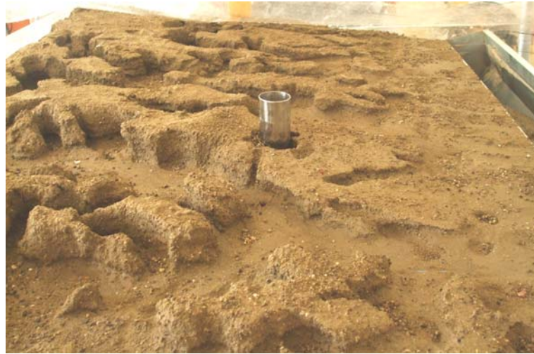
Figure 4.29. Deformed Soil Surface and Sampler in Place for Sampling
