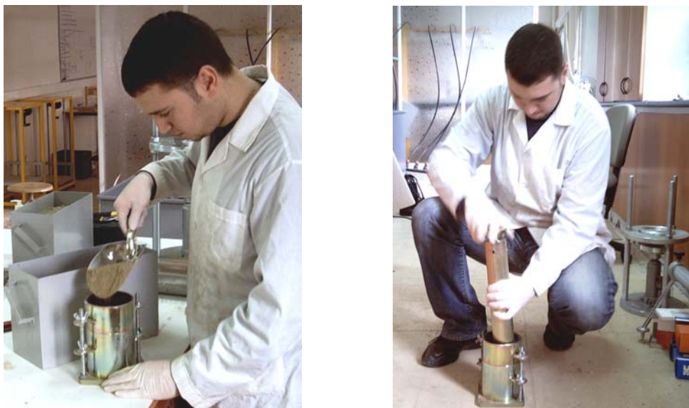
Figure 4.9. Standard Proctor Test Process
