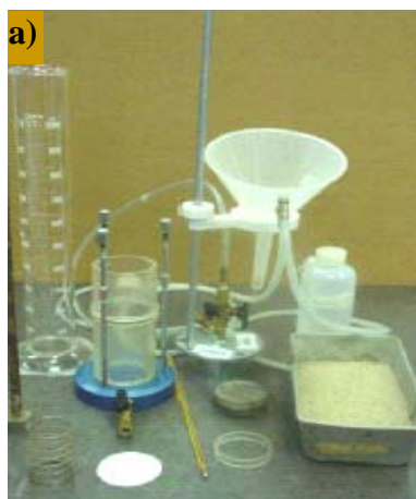
Figure 4.19. a) Falling Head Permeability Test Equipments, b) Soil Mold
