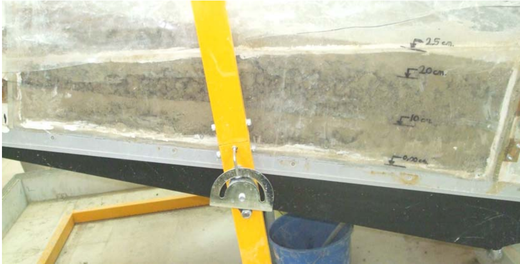
Figure 5.7. Lateral View of the Soil Slope Sample in Experiment 3
