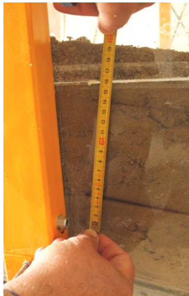
Figure 5.10. Infiltration Depth after the Experiment 5
