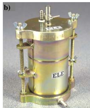
Figure 4.19. a) Falling Head Permeability Test Equipments, b) Soil Mold
