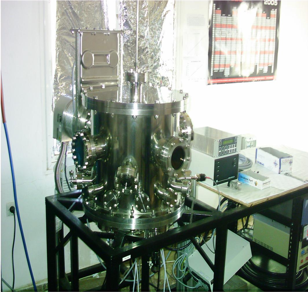
Figure 3.3. The photograph of sputter system in our laboratory
