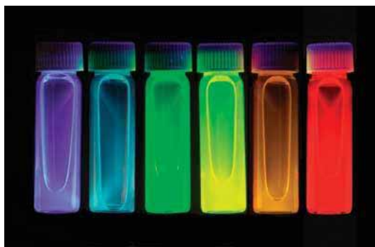
Figure 1.1. Vials of fluorescent CdSe QDs dispersed in hexane illustrate the effect of quantum confinement, in which emission wavelength depends on the size of the QD. A UV lamp serves as the excitation source. Quantum-dot sizes range from 2 nm (blue) to 8 nm (red) from left to right. (Source: Dabbousi, et al. 1997)
