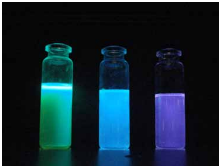
Figure 3.10. Luminescence image of CdSe x S 1-x nanoparticles under UV lamp
