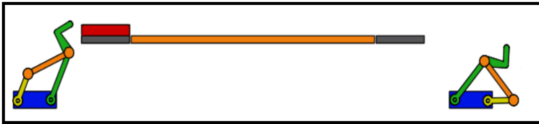
Figure 6.8. Double Four-Bar Mechanisms.
