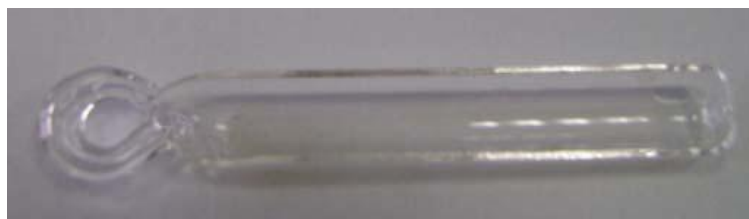
Figure 4.2. Quartz boat used to carry catalyst particles into furnace
