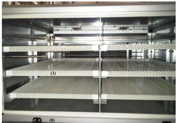
**Fig. 29.4** A view of drying trays
