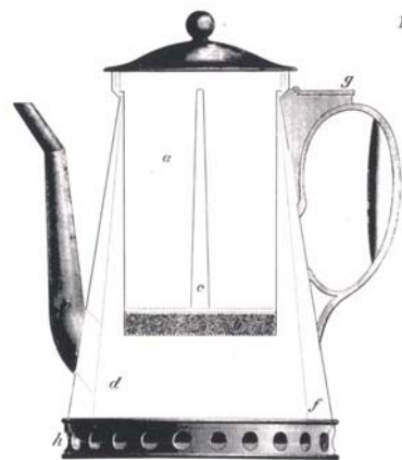
Figure 3.25. Section drawing of Rumford pot (Source: Bramah E. and Bramah J. 1995)
