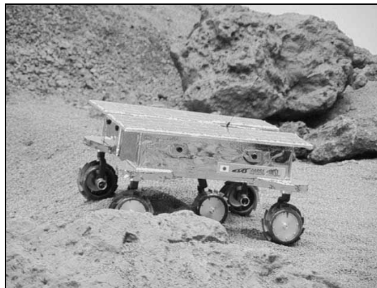
Figure 1-8: Micro5 rover with suspension named Pegasus (Courtesy of Meiji University – Japan)
