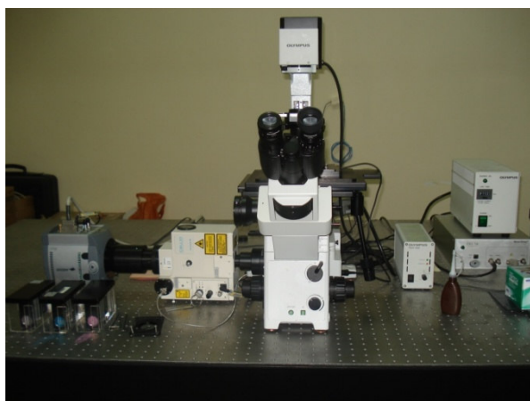
Figure 3.4. The confocal microscope used in this study (Andor Revolution).
