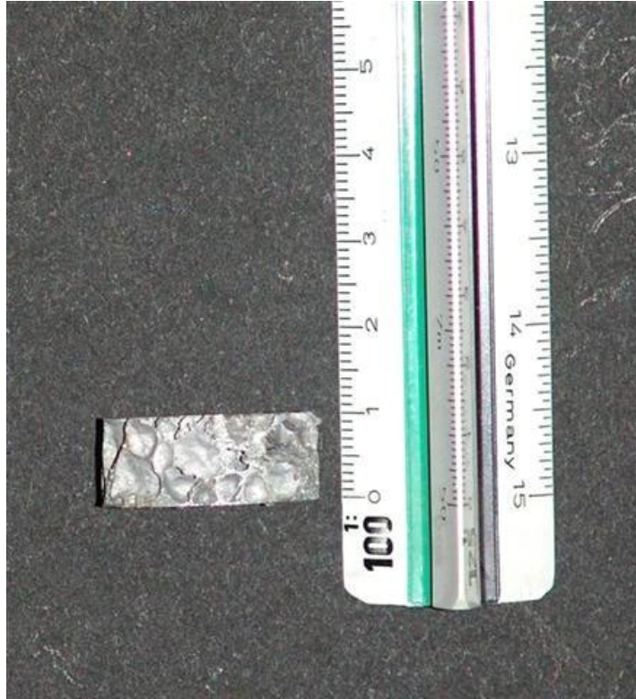
Figure 6.7. Cylindrical foam sample for sound absorption test.
