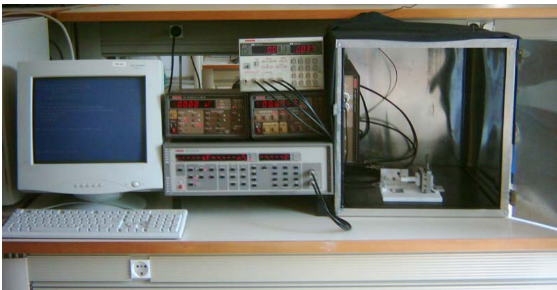
Figure 2.2 Simultaneous Capacitance-Voltage (C-V) Setup
