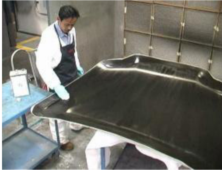
Figure 4.18. An open mould example (Source: WEB_9)
