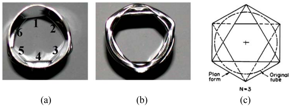
Figure 4.18 a) Top and b) bottom views of the crushed 16 mm Al tube and c) schematic view of the diamond collapse mode with 3 circumferential lobes (only figure 4.18(c), [38]).
