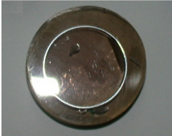
Figure 3.7 Metallographically prepared hardness test sample (6063 Al).
