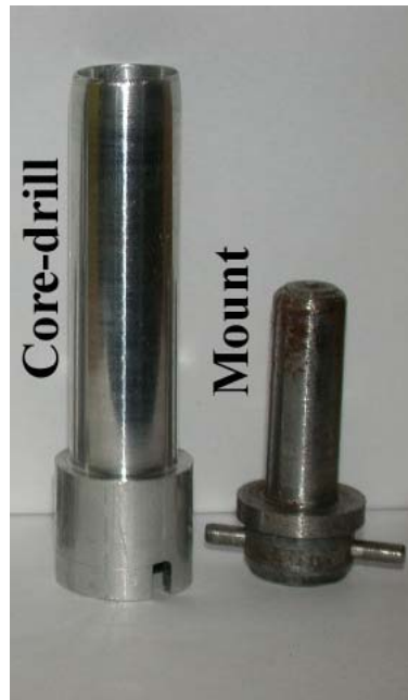
Figure 3.8 Apparatus used to core-drill cylindrical foam filler.
