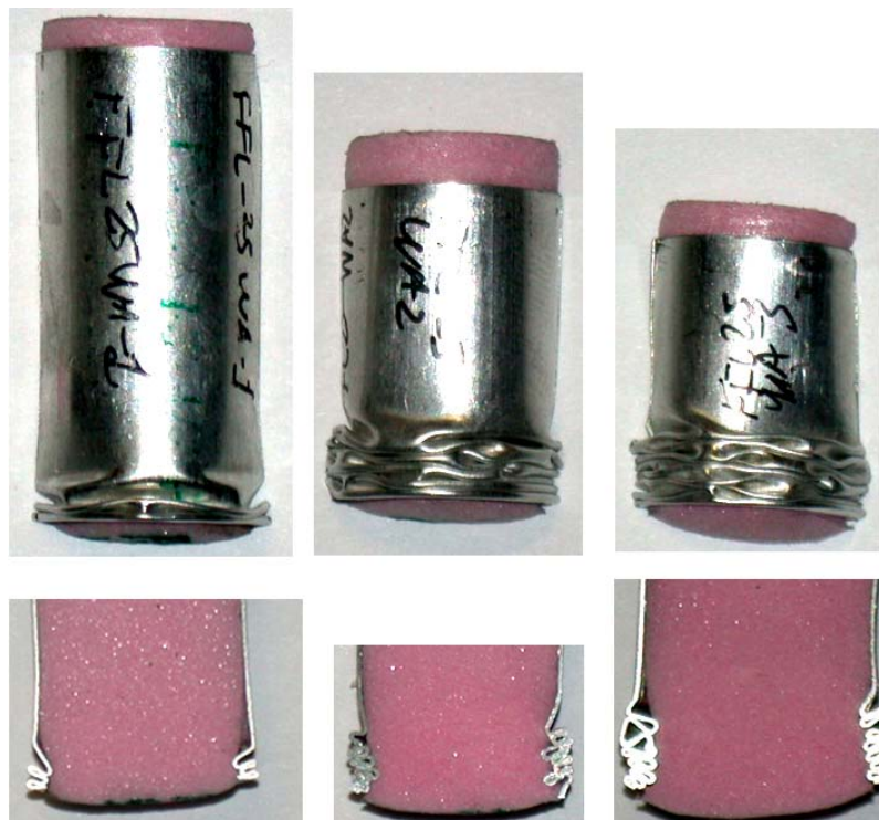
Figure 4.35 Side and cross-sections of the foam-filled 16 mm Al tube without adhesive.
