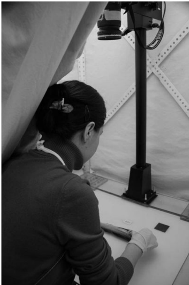
Figure 1—Light box and digital camera used to capture images. The fish and the reference square are also shown.
