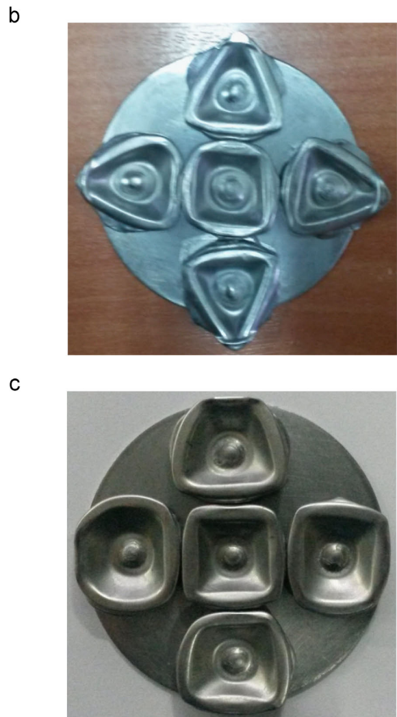
Fig. 7. (a) Comparison of unconfined and confined quasi-static crushing test results, deformed top views of (b) unconfined, and (c) confined specimen.
