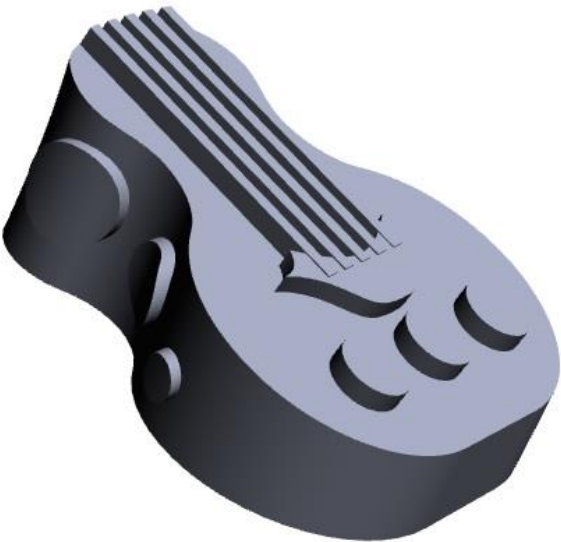
Figure 50: 3-D Box Design for the 3-INput Pre-Amplifier [11]
