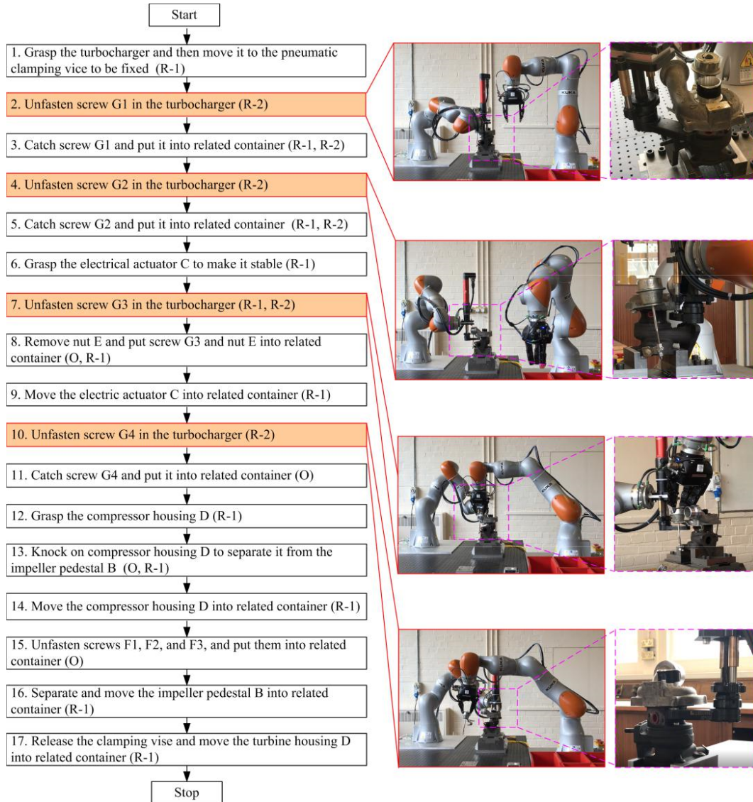
Fig. 19. Flowchart of the turbocharger disassembly operations.
