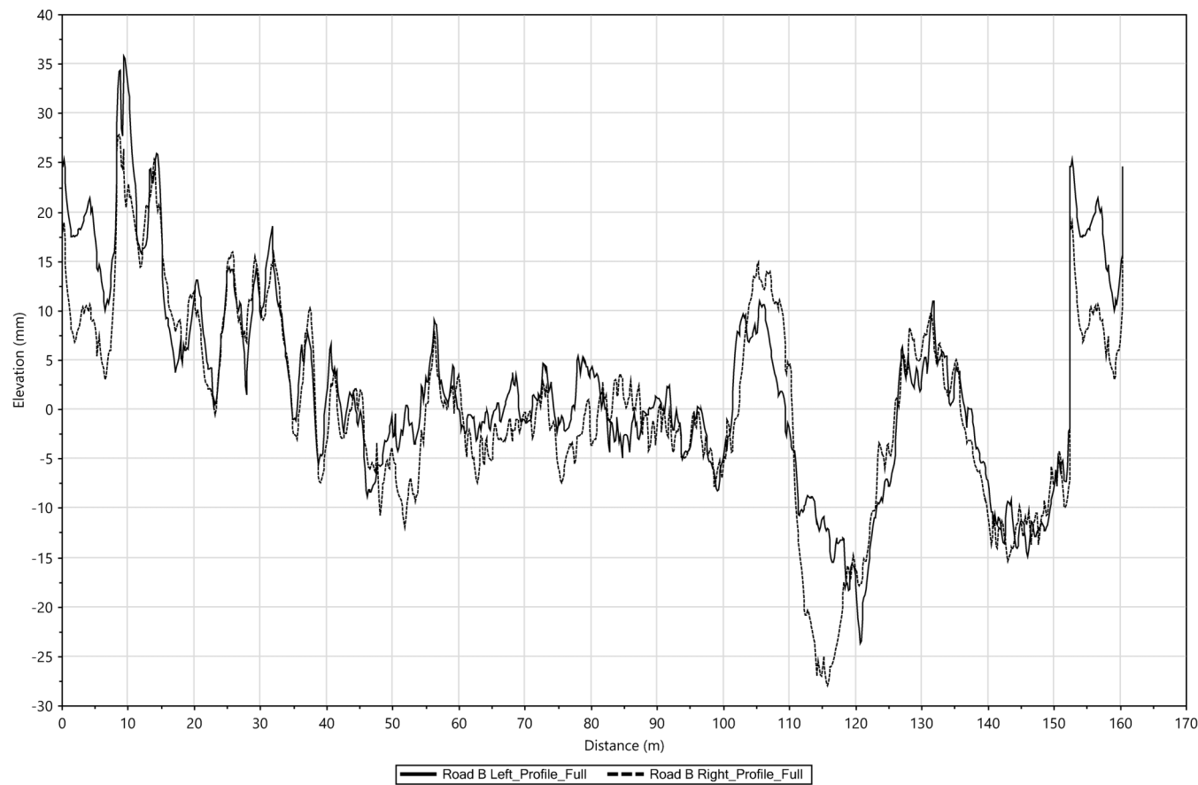
Fig. 4. Road profiles of Roads A and B.
