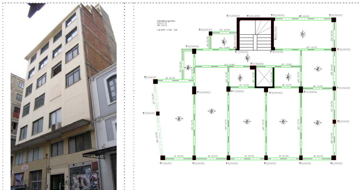
Figure 1(a). Existing multistorey RC building in the city of Thessaloniki, (case study).
