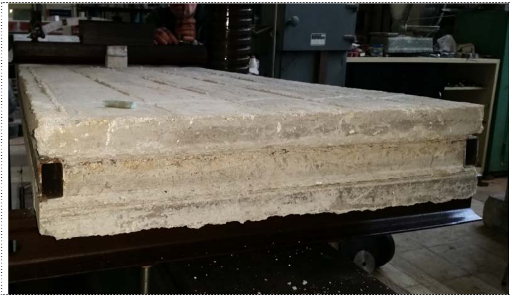
Figure 2. Elementary module of double-shell composite wall on the test bed (real size).
