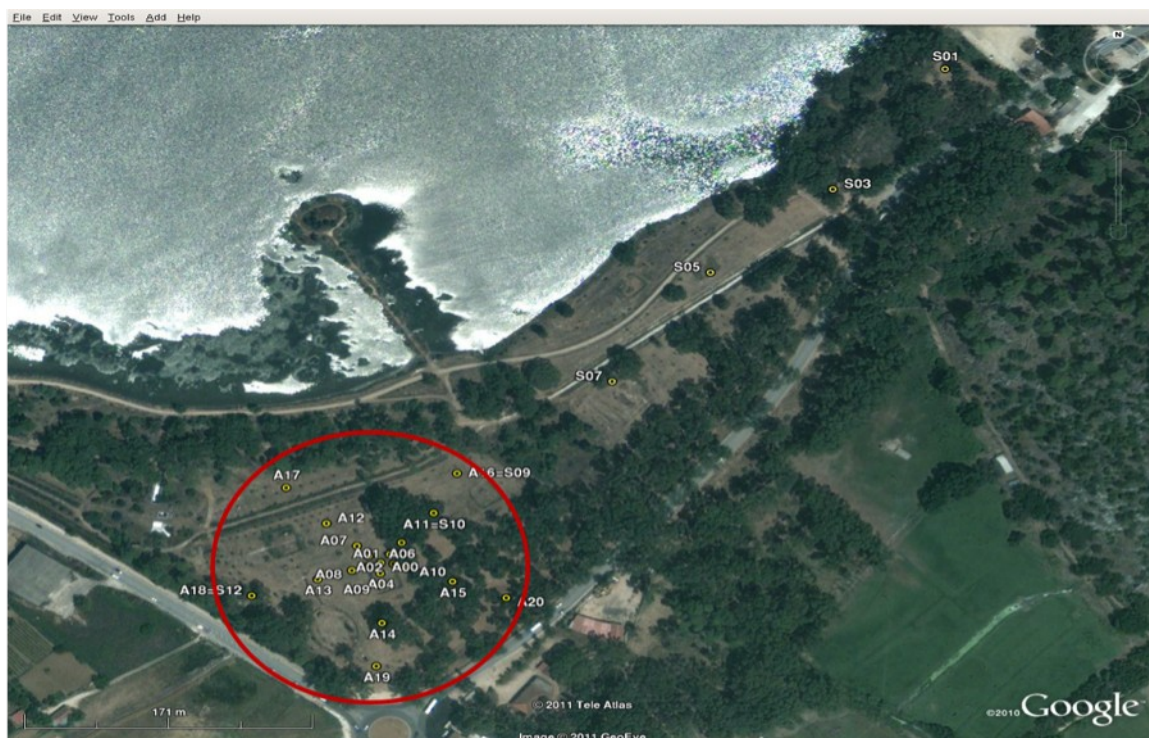
Fig. 8. Zoom in the center of the Argostoli basin array, showing the "radial array" with an aperture of 160m.
