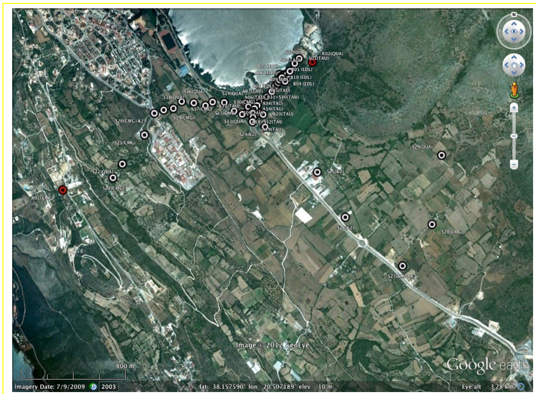
Fig. 7. Plan view of the Argostoli basin together with the seismological array configuration (red points: reference rock stations).
