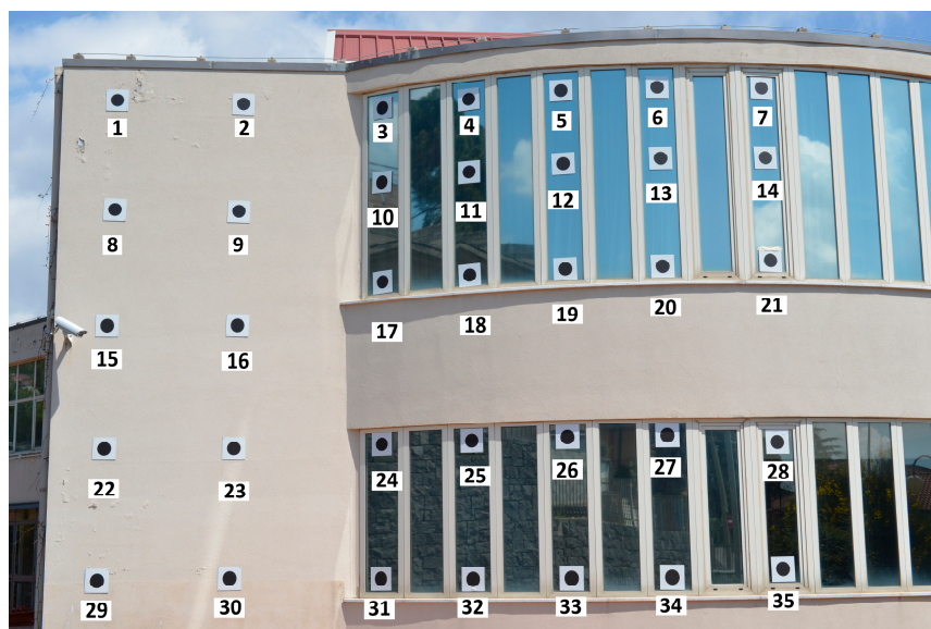
Figure 4. View of the 3D calibration test field devised on the INGV facility edifice in Nicolosi (CT). The thirty-five regularly distributed artificial targets are 0.15 m diameter black circles drawn inside white squares.
