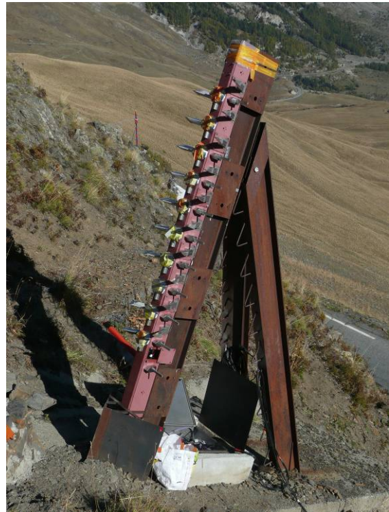
Figure 5. Tripod set in avalanche path n°2 holding velocity sensors, pressure sensors and height sensors.
