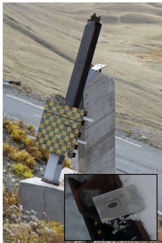
Figure 11. The instrumented structure set up in path n° 1: the beam and the 1 m 2 plate system whose loading is used to reconstruct impact pressure from avalanches. The insight is a velocity sensor set up on the hillside of the plate.
