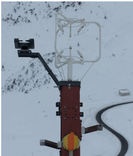
Figure 9. Snow particle counter (on left) and ultrasonic anemometer (at center) set up on top of the tripod in path n°2.
