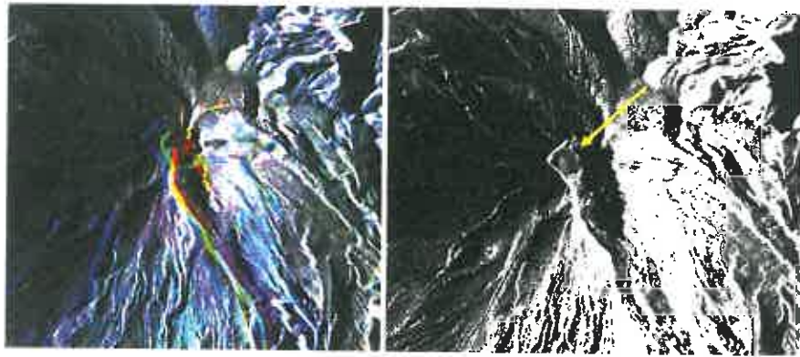
Figure 5: Left image: Multi-temporal analysis in RGB component: R= 1/5/2010, G=31/10/2010, B=8/11/2010. Evolution of the opening from 1 st May 2010 (red line), 31 st October 2010 (green line) and 8 th November 2010 (blue line), after the big event on 5 th November. Right picture: Onset of a new dome (yellow arrow)
