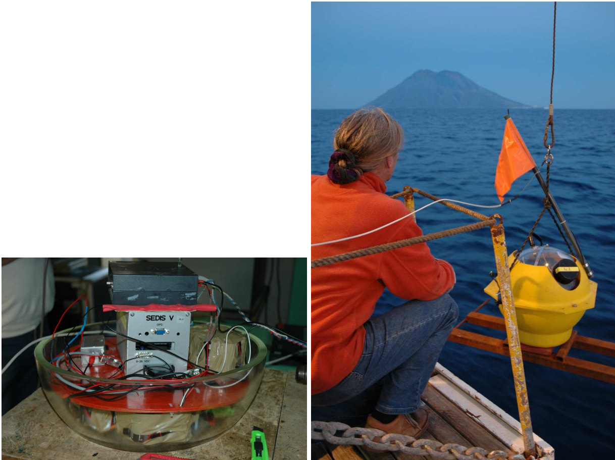
Figure 15: R/V Urania : (left) Assembling of an OBS inside a 17'' glass Benthosphere; (right) Release procedure of an OBS off Urania .
