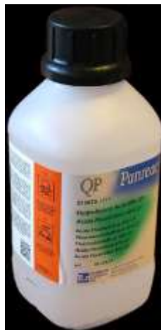
Gambar 5.5. Cairan asam Hidrofluoric yang bening justru aman disimpan di botol plastik. (Sumber https://ehs.ucsc.edu/lab-safety-manual/specialty-chemicals/hydrofluoric-acid.html )
