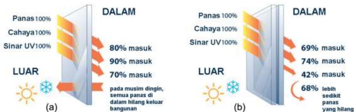
Gambar 2.34. Skematik perbandingan kaca biasa (a) dan kaca low-e (b). (Sumber http://www.firstwindows.co.nz/glass-options/product/33/clear-glass-and-low-e-glass )
