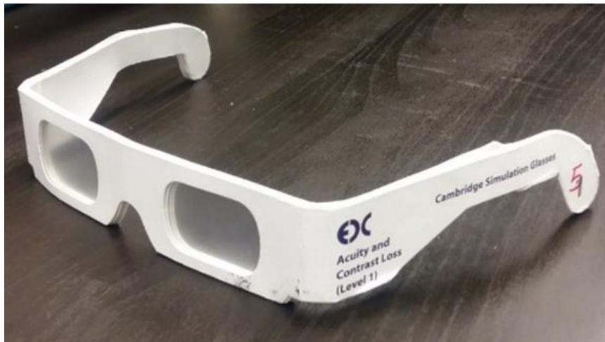
Figure B-1: One of the Cambridge simulation spectacles (level 5) used in the studies.
