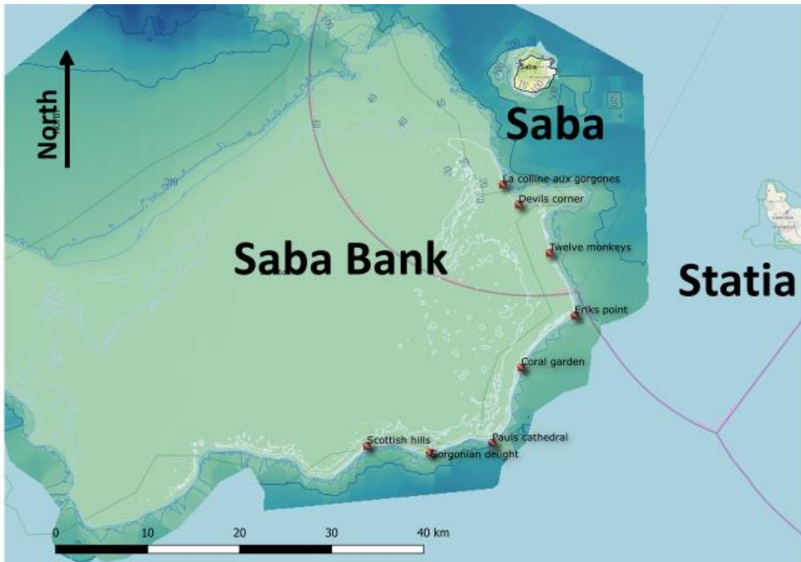
Figure 3. Bathymetry of the Saba Bank with isobath depth contour lines (Data from the Netherlands Hydrographic Service), the islands of Saba (Northeast of the Saba Bank) and St. Eustatius (East of the Saba Bank) and the 11 stations which were surveyed (Beek and Meesters 2014). Fore-reef stations were in the 17-32m depth range and the patch reef on top of the Saba Bank, Tertre de Fleur, is at 15m depth.
