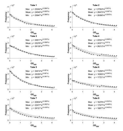
Figure 7.4: Calibration curves for cell density. The non-linear fitted exponential relationship between the frequency measured and cell density, by standard at  $OD_{600}$ , was determined using a series of cultures of P. putida KT2440 wild type with known cell density. Frequencies were first corrected with no-light measurements before calibration. The fitted lines were used to extract the formula required for translation of data to cell density. Per tube, a separate standard curve was prepared.
