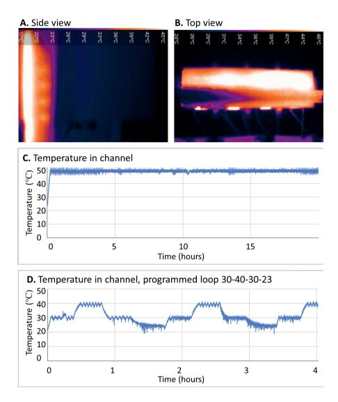
Figure 7.3: Temperature stability within the millifluidics device A) Thermal camera image of the side view of the millifluidics channel. B) Thermal camera image of the top view of the millifluidics channel. C) Temperature in channel as determined with the thermistor at output when the temperature is set at  $50^{\circ}$ C. D) Channel temperature as determined with the thermistor at output when the temperature regulation is set to a loop of  $30 - 40 - 30 - 23^{\circ}$ C.
