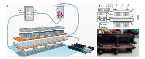
Figure 7.1: Schematic overview of millifluidics device A) depicts the millifluidics device, 1. the PDMS gel through which eight microchannels run. 2. Top Peltier elements, in charge of cooling the system. The fans are placed on top for heat dispersion. 3. Bottom Peltier elements, for heating the system. 4. Thermistor for temperature registration, which via the Arduino Uno is then used to regulate the Peltier elements, placed within the bacterial sample where the PDMS meets the tubing.
