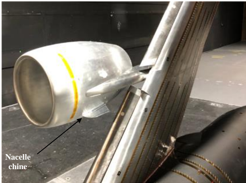
Fig. 19. Nacelle chine installed on the inboard side of the engine nacelle.
