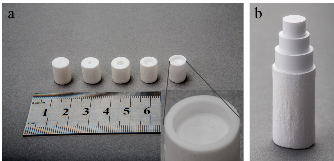
Fig. 5. Photograph of (a) sintered alumina samples that were drilled with (from left to right) 1.1, 2, 4, 6, and 8.2 mm drill bits before sintering, (b) a green body after lathing.
