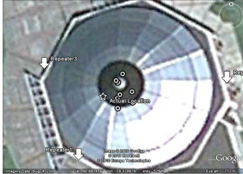
Fig. 13. 2D indoor positioning experiment results imposed on the satellite image of the Dining Hall at Sabanci University. The dome shaped metallic structure of 43 m diameter blocks GPS signals.
