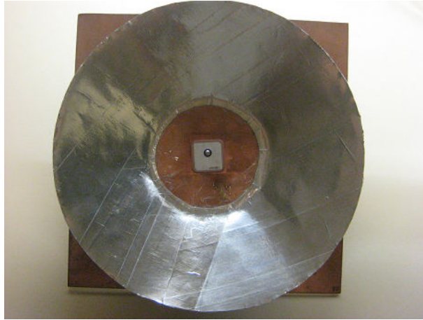
Fig. 5. A standard GPS antenna and an aluminum conical reflector forming the directional GPS antenna. The measured beamwidth of the structure is 60^\circ .
