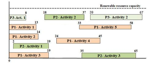
Figure 5.2: Gantt chart of a sample schedule generated as an output of the holistic approach
