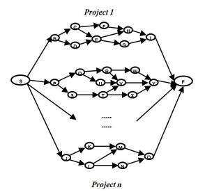
Figure 3.1: Composite multi-project network with N projects and dummy start-finish nodes
