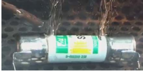
Fig. 1 Littelfuse SPF 10 amp fuse gross leak test showing a steady stream of gas bubbles at the interface of the fuse body and metal caps.
