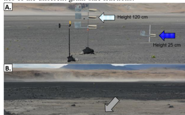
Figure 1: Wind-blown dust in field work area, Iceland. A. Dust collectors (at 120 cm and 25 cm high) & anemometer. B. Arrow shows deposits sourcing the dust.
