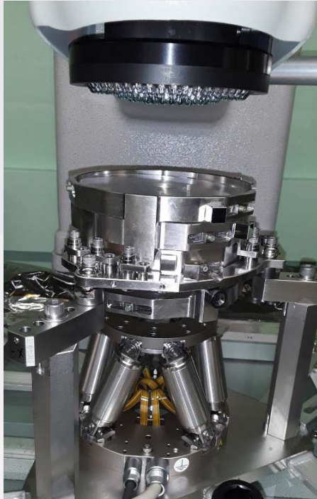
WFIRST Grism Engineering Design Unit on flexure legs while modifying alignment
