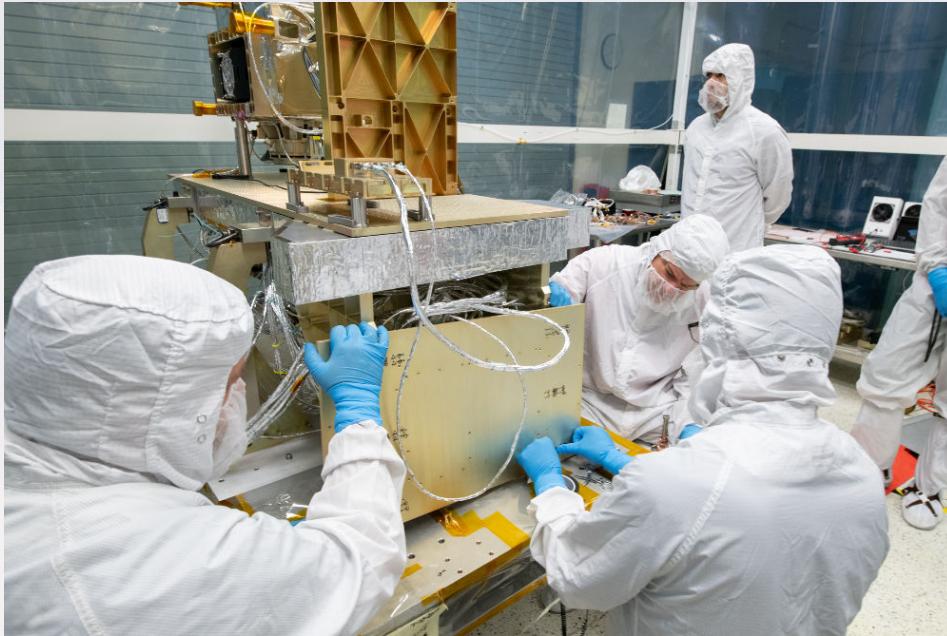
DAU de-integration/removal from the Functional Bench; OCI ETU FlatSat End-to-End Electrical System Test – Electrical Integration
