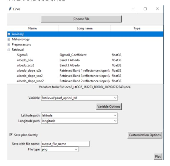
The internal use case provides a way to plot previously downloaded files through a graphical interface or through the command line, with options to customize output, plot limits, geospatial projection, plot titles, color mappings and displays, and value ranges.
