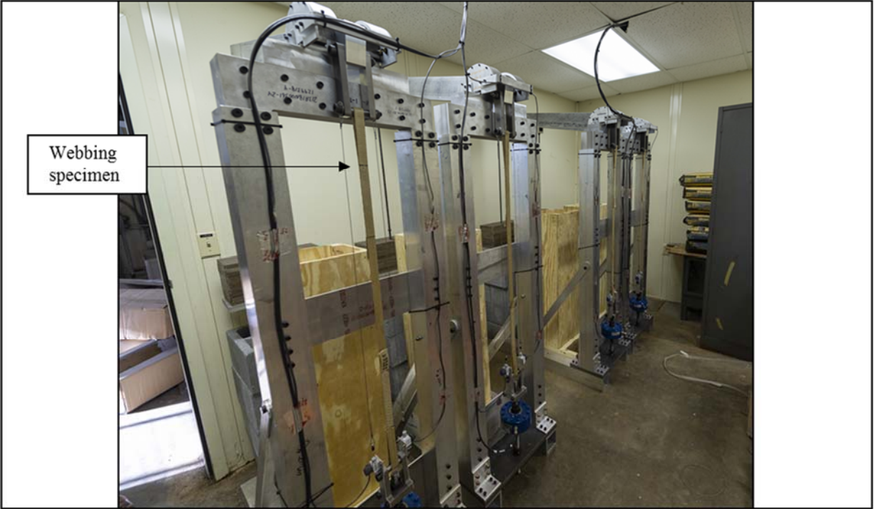
Figure 7. Four low-cost small-volume lever-arm creep test stands in room A.
