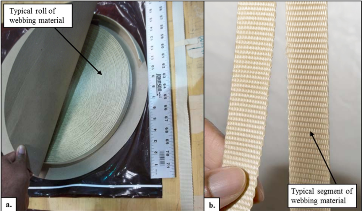
Figure 4. Vectran webbing material, (a.) typical roll and (b.) webbing segment.
