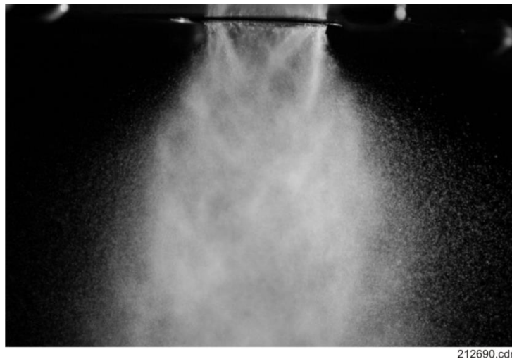
Figure 8-5. CRESS Spray Photograph at Simulated 85 Percent Condition
