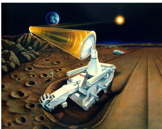
Figure 31. Automated Mark II Lunar Miner for Extracting He-3 and SWI Volatiles [75]
