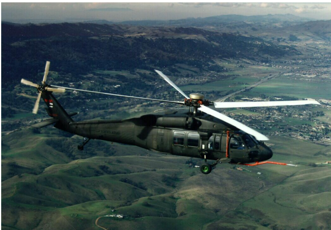
Figure 1. UH-60A with instrumented blades flying over the San Joaquin Valley during the UH-60A Airloads Flight Test Program.
