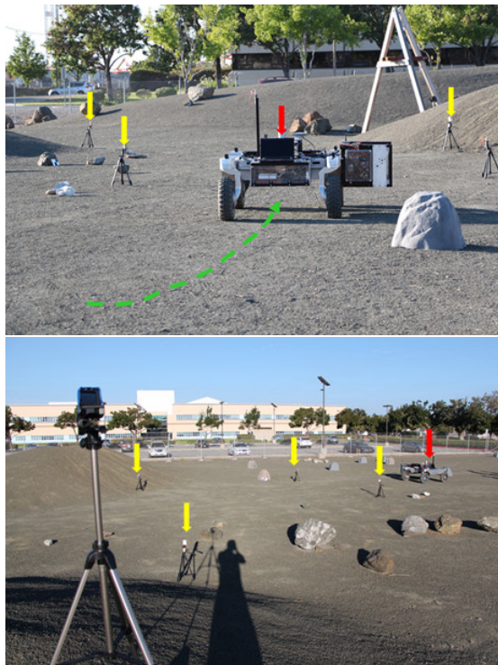
Figure 14. Outdoor multi-node field test setup with mobile rover node. In this particular test, nodes were manually placed on tripods so ground truth positions could be surveyed and range measurements could be isolated from terrain interference.
