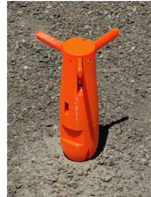
Figure 15. Recent miniaturized dart projectile enclosure emplaced during field test.
