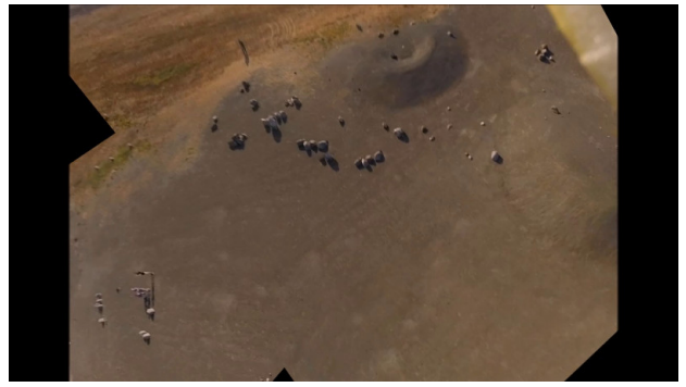
Figure 11. Synthetic overhead view generated from mosaic of images collected while in flight.
