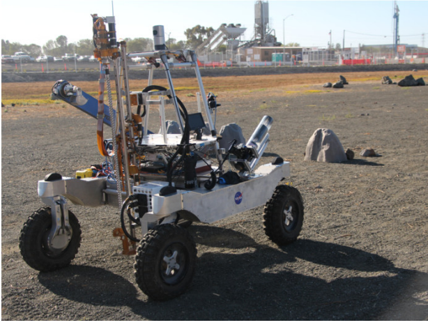
Figure 6. Projectile launcher mounted to K Rex2 test rover.
