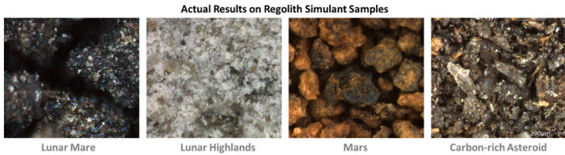
Figure 12. Image samples recorded from the miniature solid-state 3D microscope on varied samples. Captured at 1\mu\text{m}/\text{pixel} .
