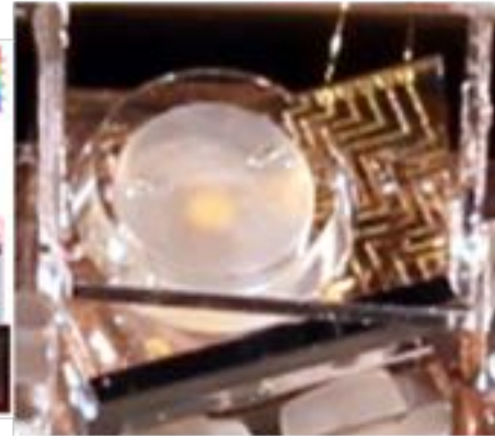
Resonator with PZT
