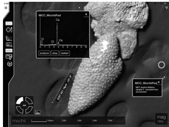
Figure 3. Spectroscopy and image of sediment particle gathered on EVA and analyzed in-situ in the underwater Aquarius habitat by NEEMO XXIII crew member J. Watkins. Some sediment contained calcium carbonate from deceased organisms, whereas others (not shown) were silicate-based.
