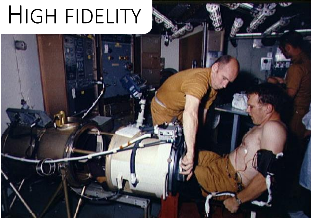
SKYLAB Medical Experiment Altitude Test (SMEAT) (56 Days) Atmosphere 70% O 2 at 5 psia Textiles: Apparel, sleeping bags, pillows, curtains, towels
