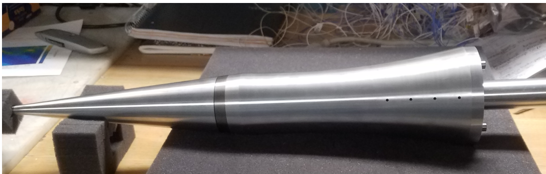
Figure 17. Photograph of cone-flare model with dummy suction section
